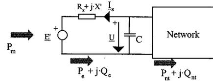
Fig. 2. Dynamic model of an asynchronous generator.
