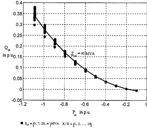
Fig. 4. Variables  $P_{nt}$  and  $Q_{nt}$  under several steady-state situations.
