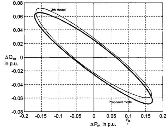
Fig. 7. Comparative results of power fluctuations between third-order dynamic model and proposed model  $P_{nt,0} = -0.992$  p.u.,  $Q_{nt,0} = 0.2786$  p.u.
