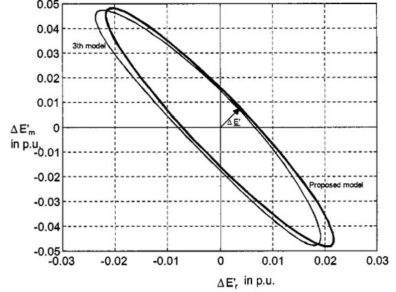
Fig. 6. Comparative results of internal voltage fluctuations between third-order dynamic model and proposed model  $\underline{E}_0 = 0.8521 + j0.2489$ .
