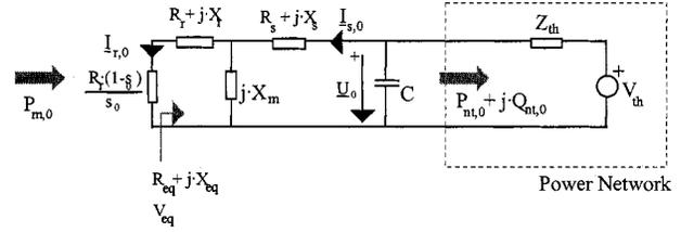
Fig. 10.  $RX$  model of the asynchronous machine in the network.
