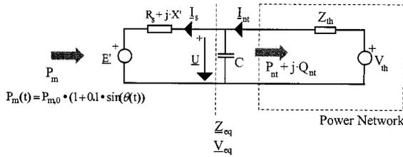
Fig. 3. Asynchronous wind energy converter.
