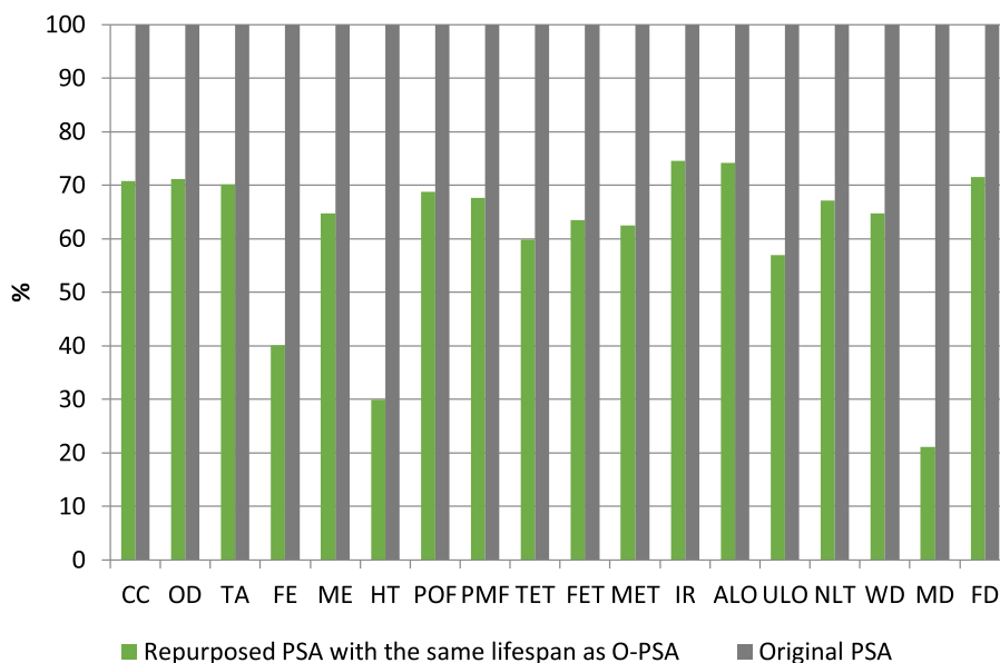
Fig. 5. Sensitivity analysis results when considering the lifespan of the R-PSA equal to that of the O-PSA. Recipe Midpoint (H), characterization.
